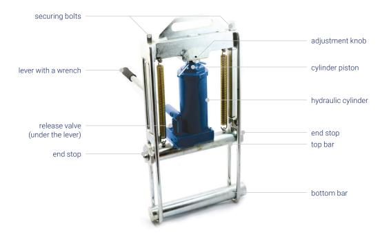
A hydraulic pipe squeeze-off tool allows you to manually / hydraulically clamp polyethylene pipes to temporarily shut off the flow of medium inside a pipeline. When using the tool, follow the health and safety rules.
